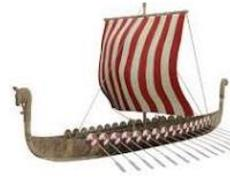
**Longships** were vessels made and used for trade, exploring, and raiding. It was the Vikings who mastered the design of light fast longships that could also go up rivers. Longships were clever in that they used **both wind propulsion and rowing power**. They had a sail and a mast, but also had oars for rowing in case the wind disappeared.
